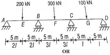
4 Using flexibility matrix method for the beam shown below and draw shear force and L3 12M bending moment diagrams, EI is Constant.
